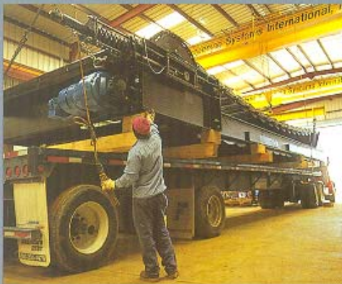
Reassembled traveling water screens are carefully checked and test run before being returned for reinstallation.
